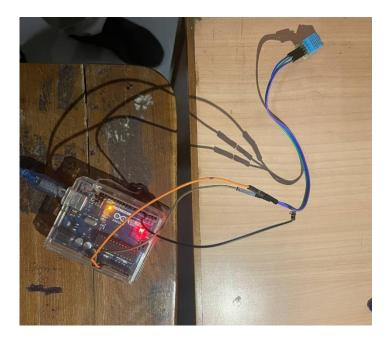
DHT11 sensor to detect Humidity and Temperature
